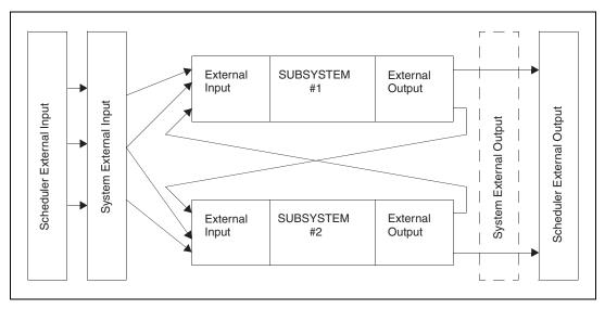
Figure 5-1. Interface Layering Diagram
